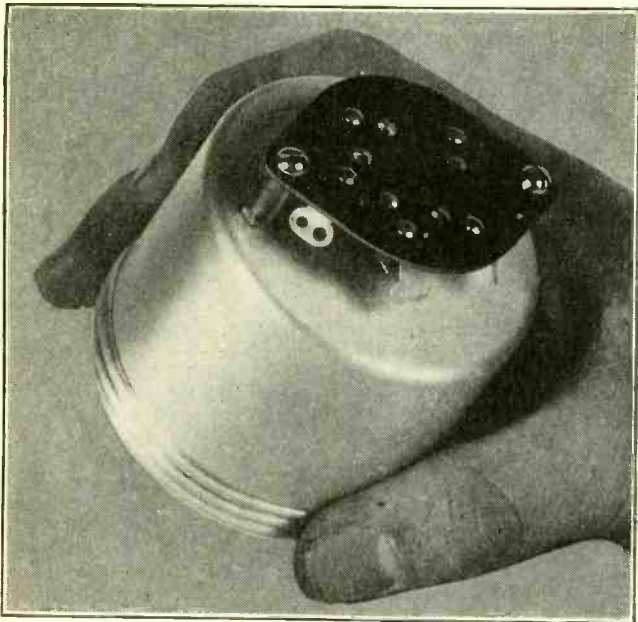
Fig. 2 Appearance of the shielded intermediate frequency transformer, with socket affixed to the screw cap
